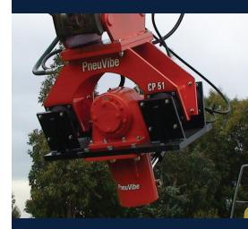
With clamping devices you can effectively combine sheet and perform pile driving in certain soil conditions.
