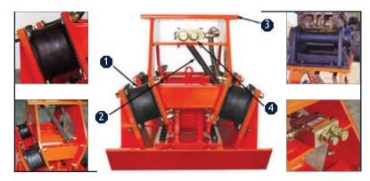
PneuVibes patented system ensures increased elastomer life and minimises vibration transmitted to the boom, thus reducing wear on the pins and bushes of the excavator.
