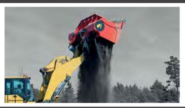
With ALLU you can process different materials such as topsoil, black top and dirt, excavated and waste soil, contaminated soil, clay, peat, bark, compost, bio waste, demolition waste, construction waste, milled asphalt, glass, coal, oil shale, lime stone and several other materials.
